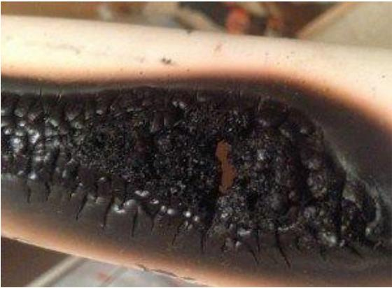
Corrosion buildup on secondary cells
