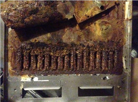
Vent pipe damaged from heat
